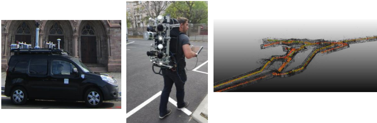
Figures. Mobile mapping system development platform at IGN and the digitization of sewers.
