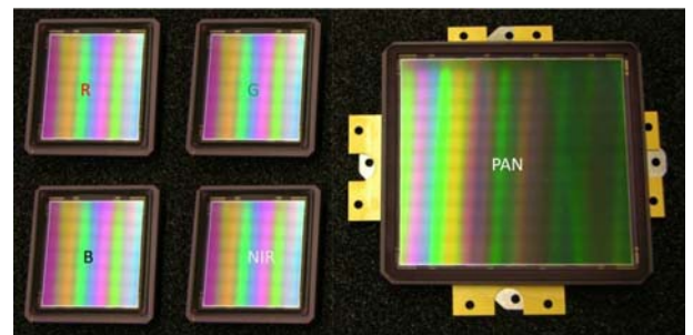
Figure 2: CCD frame sensors from DALSA used in the DMC II camera set-up. The large format monolithic 250 MPix pan-chromatic chip (right) and the smaller format 40 Mpix CCD frames (left), where one is used for each of the four MS bands. (© Neumann, 2011).
