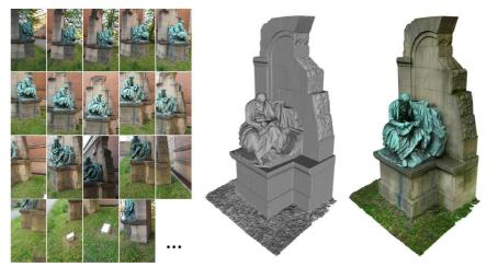
3D reconstruction from imagery: given a set of input images (left), the main objective is to derive a 3D scene representation in terms of geometry and color information
