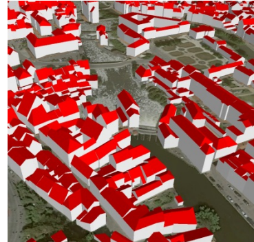
Figure 2: Reconstruction of 3D Building Model (LoD2) in the historic city center of Bamberg with 2D editing window (left), 3D view with corresponding laser point cloud (middle) and visualisation of the result in CityGML combined with a DOP (right).
